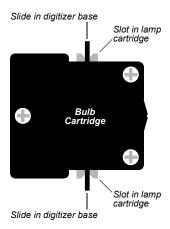
■ When the cartridge is nearly all the way in, push it firmly until you feel the connector snap into place.
