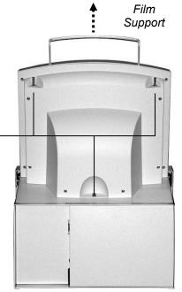
c. Lift the feeder up and off the digitizer base.
